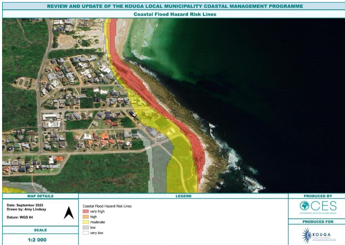
Figure 4.22: Infrastructure at Cape St Francis that is located in very high, high and moderate coastal flood hazard risk zones.
