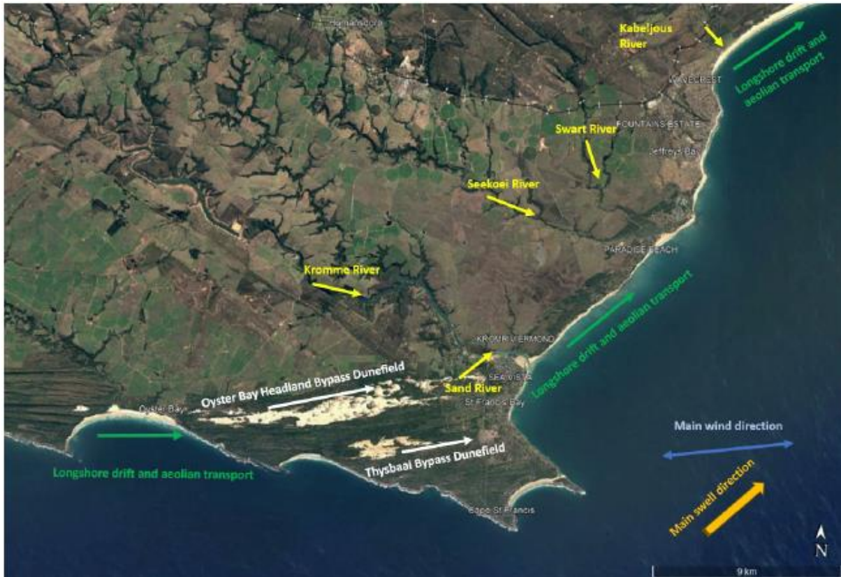
Figure 4.15: The main sediment pathways of the KLM coastal zone (van der Waal, 2024). Sediment System Modification
